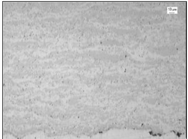
Above: Typical coating microstructure, as obtained using JK ® 112 Parameter Set B
