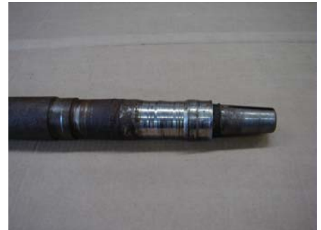
FIGURE 2: WORN SLEEVE THAT HAS BEEN TAKEN OUT OF SERVICE
