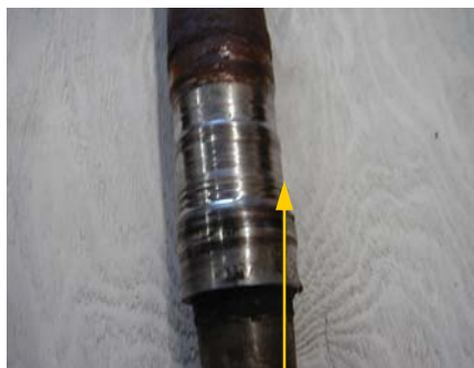
FIGURE 3: WORN AREA TO BE RE-PAIRED WITH ROKIDE C (CHROME OXIDE) COATING
