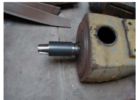
FIGURE 4: ROKIDE C COATED SLEEVE INSTALLED INTO PUMP ASSEMBLY. SLEEVE HAS BEEN COATED AND GROUND TO ACHIEVE DIMENSIONAL FIT AND FINISH
