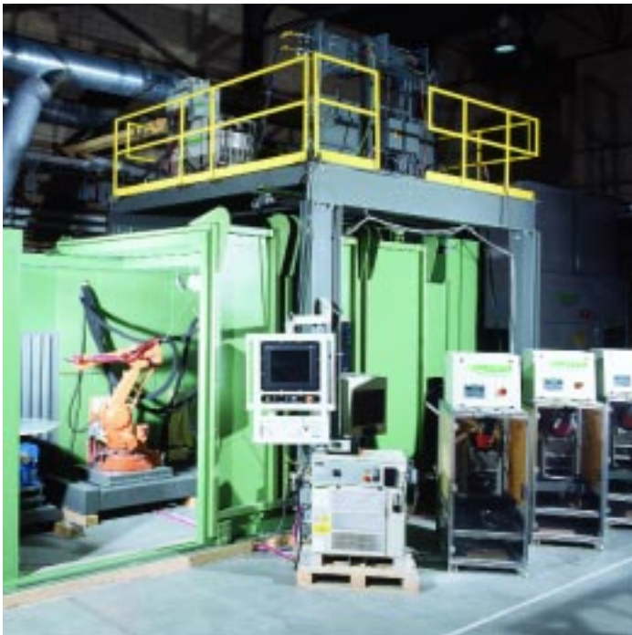
Each plasma spray system includes everything you need to produce outstanding coatings, whether your applications require a simple unit with an SG-100 gun (right) or a sophisticated, fully integrated robotic system (above).
