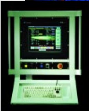
The 5501 controller housed in the Spray Process Execution Control (S.P.E.C.) Station, with separate electrical (shown) and mechanical modules.
