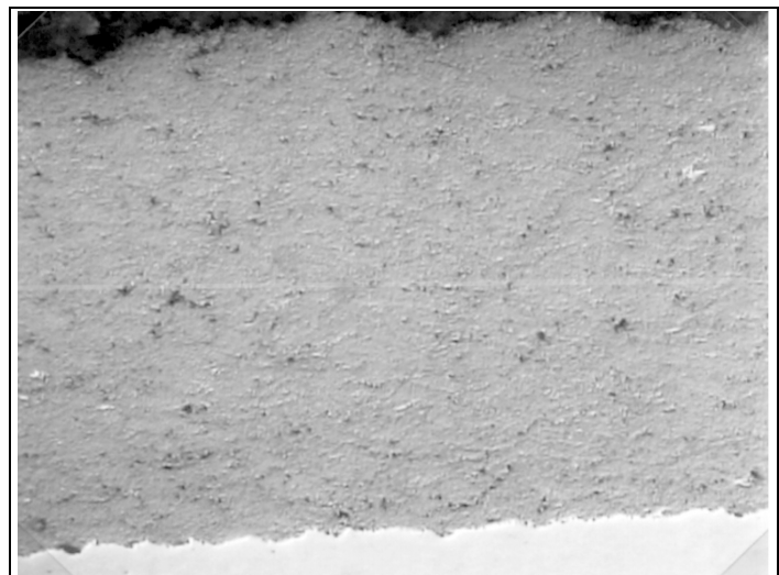
TAFE 1310VM WC – 10 Ni Coating 200X Sprayed at 10 lb/hr Etchant: None (as Polished)
