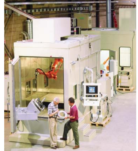
Among the advanced plasma control options available with Net Energy are the integrated PC/PLC-based Model 7700 UPC (above) and the unique Model 7700 PlazJet II, a high power plasma spray system.
